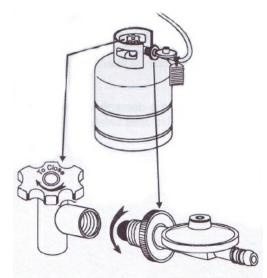
To close the cylinder valve turn the control knob fully in the direction of the arrow To engage and tighten the Regulator, turn the handwheel in the direction of the arrow
